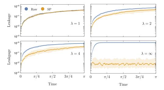
Figure 8. The leakage probability due to experimental noise as a function of time at different values of the correlation length  $\lambda$ . The simulation is repeated 100 times with different instances of the experimental noise. The solid dots represent the median of the leakage and the bars correspond to the 25%-75% percentile regions.
